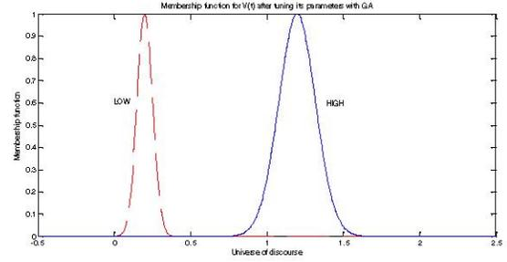
Fig.8 Membership functions for V (t) after tuning their parameters by GA.
