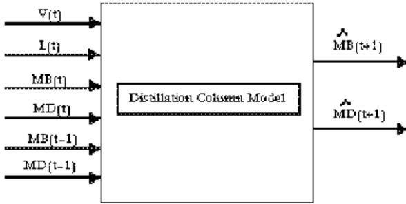
Fig.3 Block diagram of distillation column fuzzy model.
